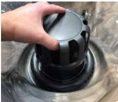
Pull Up to Remove Floater Assembly
