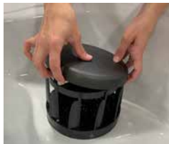
Remove Top Cap by Gently Lifting
